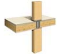
partial encapsulation during construction
