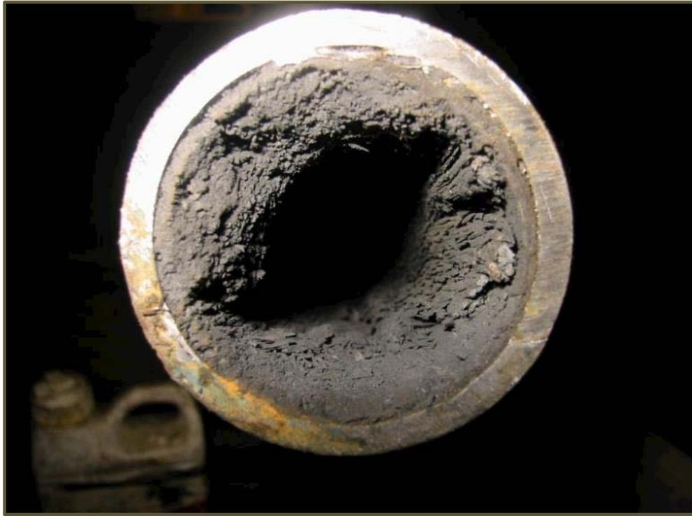
Undetected or ignored can lead to coking of oil...
