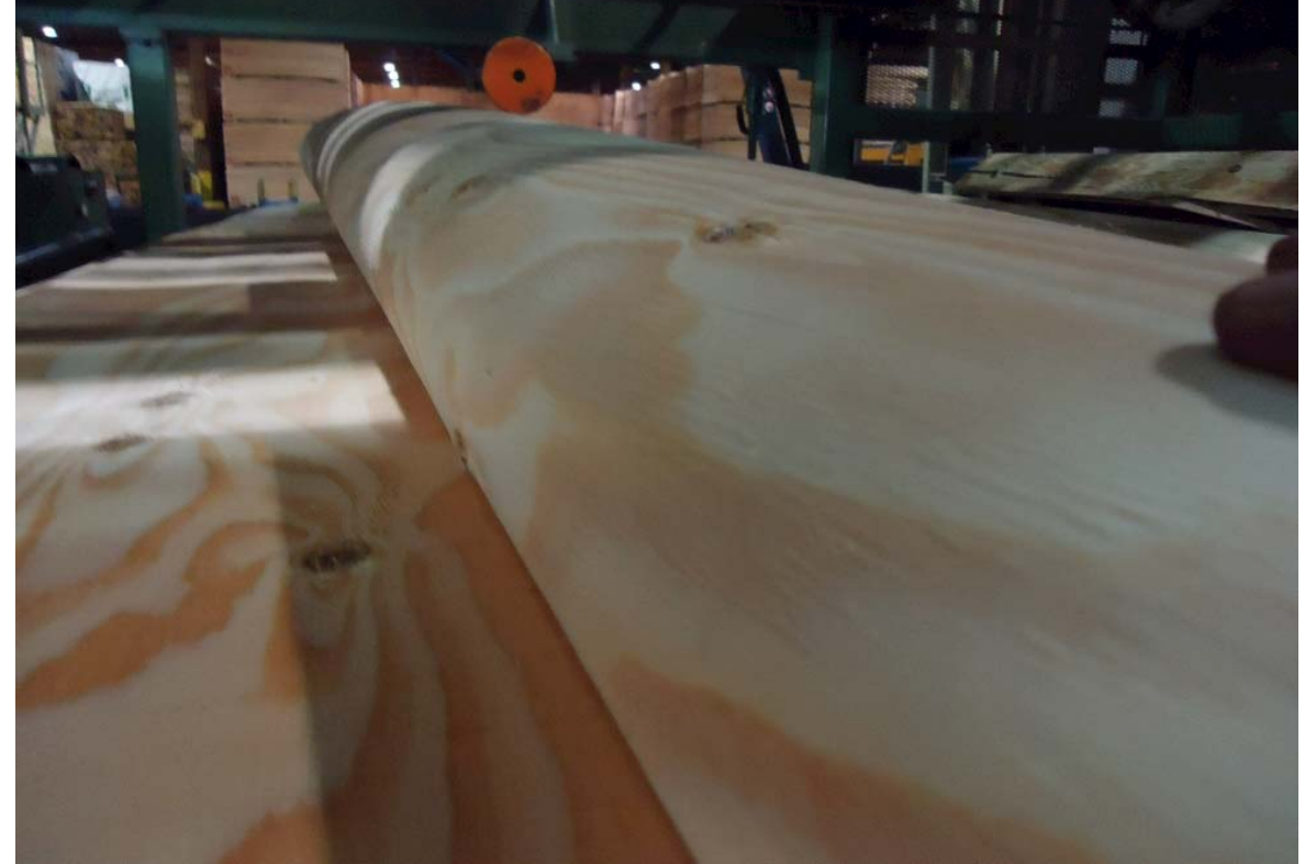
Very smooth surface with small lathe checks
