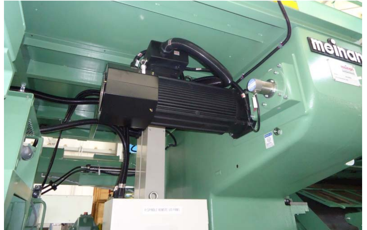
Single 30 HP AC servo motor – knife carriage
