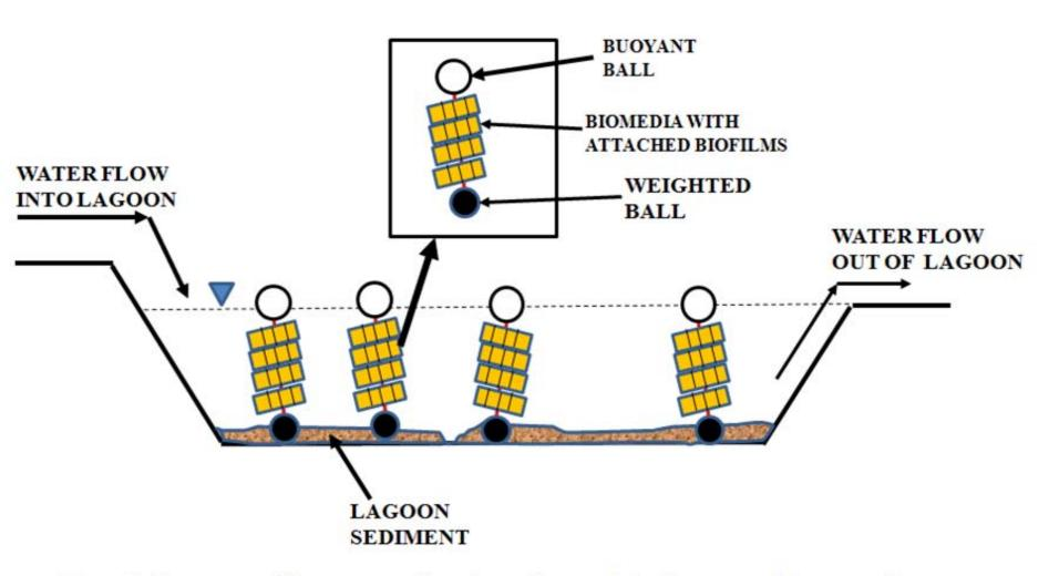
Even in lagoons with no water flow in and out of the Lagoon, this type of treatment can treat the water in-place (*in-situ*) with no water being pumped in and out of the lagoon.
