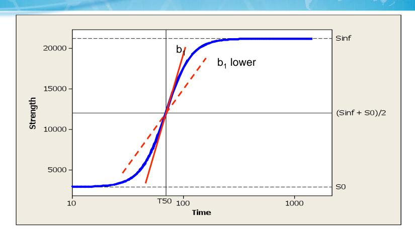
$$Strength = \frac{S_{\inf} - S_0}{1 + \exp((T_{50} + T'_{50} * (\frac{OvenT - 25}{10})) - Ln(Time)) * [b_1 + b'_1 * (\frac{WoodT - 5}{15})]} + S_0$$
