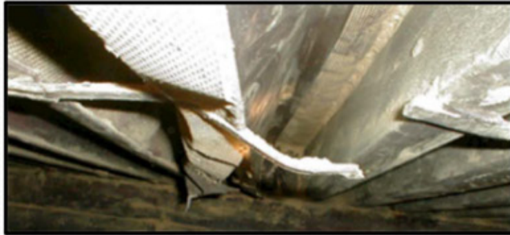
Thermal expansion not accounted for
